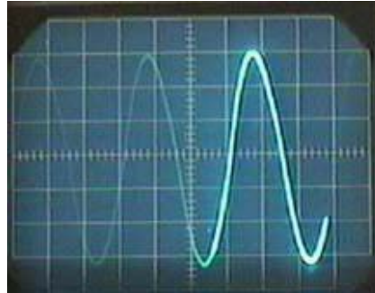
Waveform at 950 watt load.
