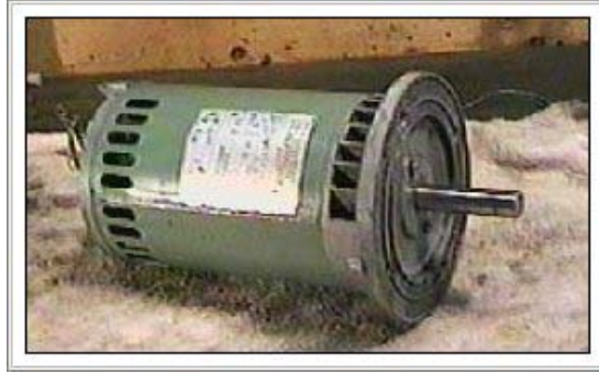
Typical waterpump motor
